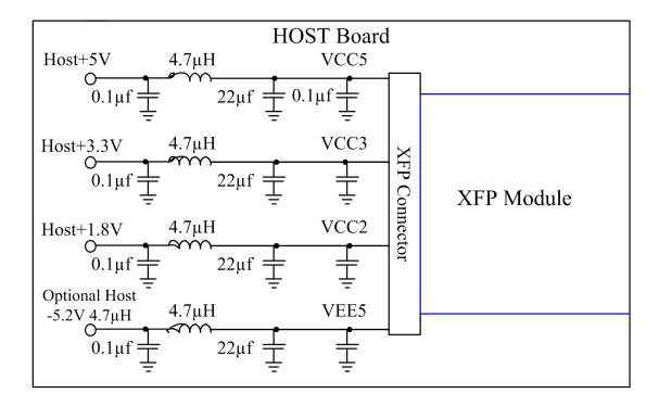
**Recommended High-speed Interface Circuit**
