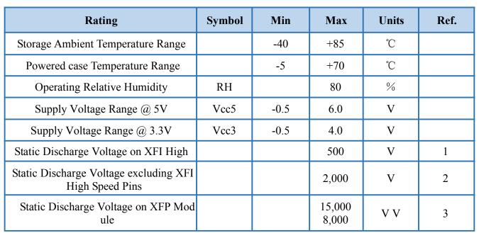
Any stress beyond the maximum ratings can result in permanent damage. The device specifications are guaranteed only under the recommended operating conditions.
